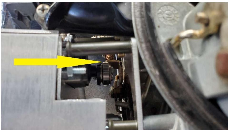
NOTE: If the idle screw does not make contact with the center of the idle servo bearing, the idle screw bracket should be bent so that it does. It can be easily bent inward with your thumb or bent outward using a flat screwdriver.
