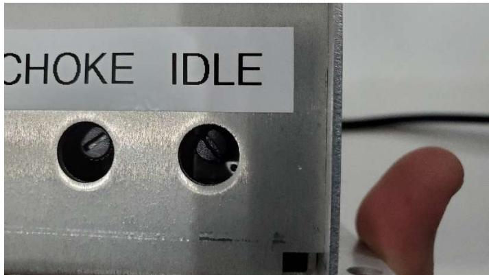
15. It is normal for the engine to not run totally smooth within the first 30 seconds however if the engine has not fully smoothed out after 30 seconds, slowly adjust the choke potentiometer one direction and then the other until the engine smooths out. Small adjustments make big differences. Simultaneously adjust the high idle potentiometer to keep the RPM at approximately 1600 RPM.
