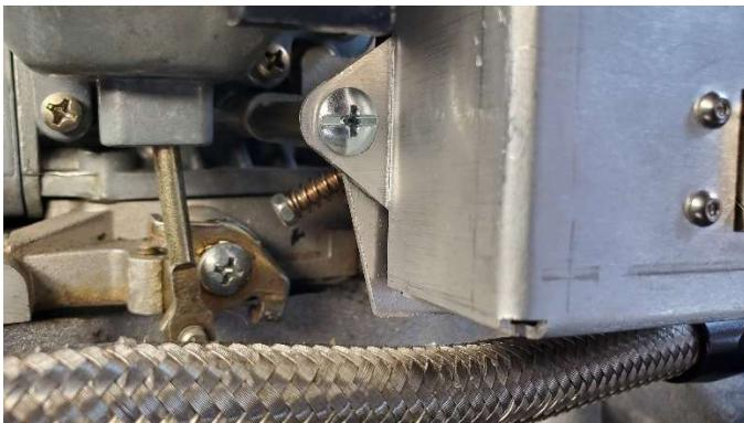
8. Turn high idle screw in until it just begins to contact the new high idle bearing. This can be felt by spinning the bearing back and forth with your finger until a slight resistance is felt. Then back the screw out 1/2 turn.
